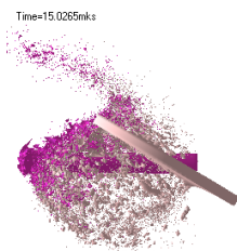
Fig. 3. Impact at an angle of 60 degrees (projectile: tungsten alloy, radius 0.2 cm, length 4 cm, a barrier: steel, radius 1.6 cm, thickness 0.2 cm, v = 2764 m/s).
