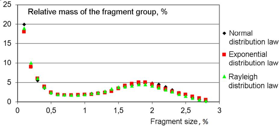
FIGURE 2. Average fragmentation spectra for different distribution laws (standard deviation 10%)
