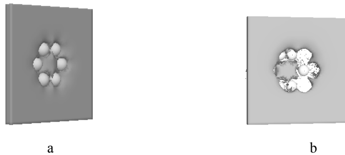
Figure 1. Group impact of compact elements with a thin target at a velocity of 800 m/s: (a) - t = 10 \mu\text{s} ; (b) - t = 75 \mu\text{s} .
